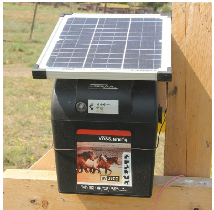
Energizer for an electric fence powered by solar energy (Hanns Kirchmeir)
